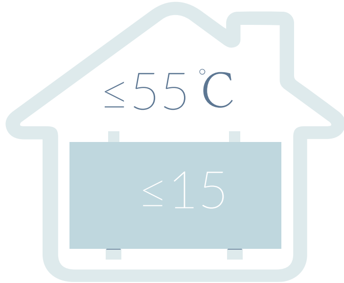
The last slabs in each rack must be kept in a position with the backside facing out. Temperatures in storage should not exceed 55 °C.
